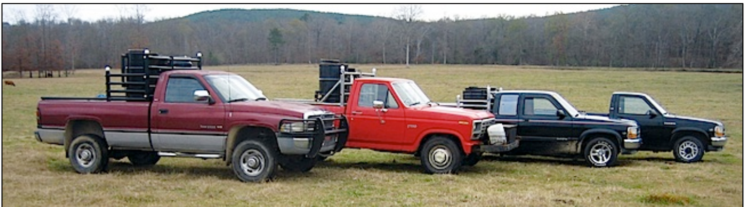
Fig. 2: Woodgas trucks, from left: '95 Dodge Ram 2500 V10; '84 Ford F250 V8; '93 Dodge Dakota V8; '92 Dakota V8 (conversion in progress)
