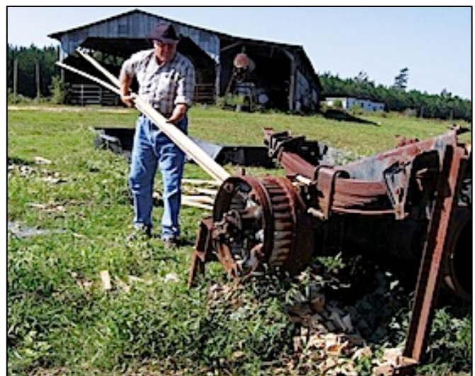
Fig. 7: Homemade "wood chucker" (made from remains of an old truck) slices scrap wood
