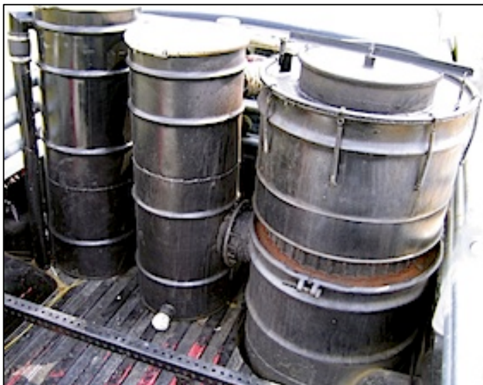
Fig. 4: from right: gasifier, heat exchanger, filter.
