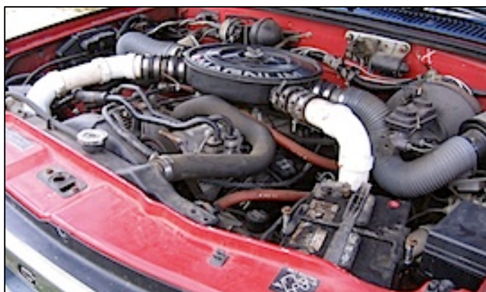
Fig. 4: PVC piping directs cooled and filtered woodgas to the engine.
