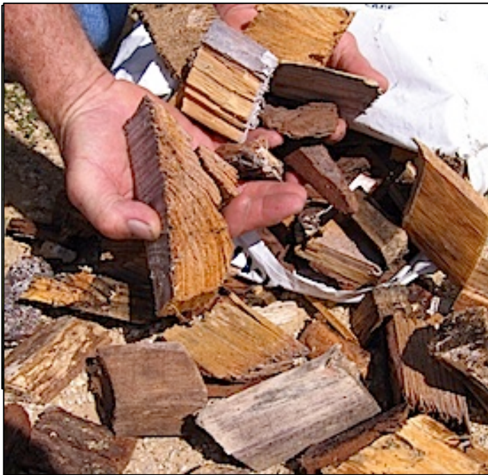
Fig. 6: Wood chunks that power Wayne Keith's trucks.
